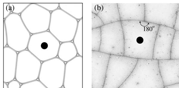
FIG. 3. (a) A detail of a dry, two-dimensional foam. The cell marked by the disk has six sides and six neighbors. (b) A detail of a hierarchical crack pattern. The marked cell has four sides, but six neighbors.
