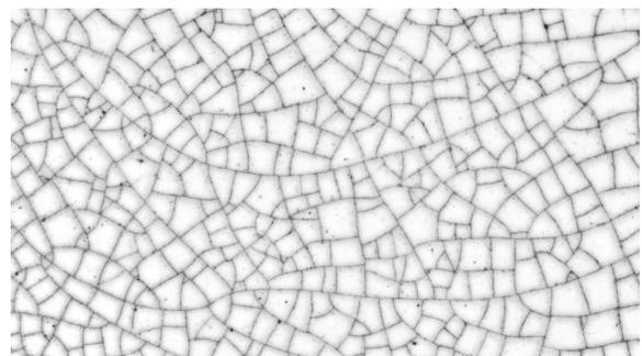
FIG. 1. A hierarchical crack pattern in the glaze of a ceramic plate. The first crack to have formed can be seen as a long sinuous line along the lower part of the photograph.
